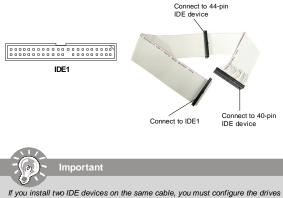
If you install two IDE devices on the same cable, you must configure the drives separately to master / slave mode by setting jumpers. Refer to IDE device's documentation supplied by the vendors for jumper setting instructions.
